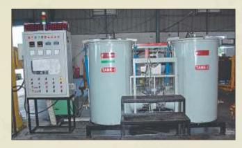
**Diamond Delta** ( $\Delta$ ) chains are vacuum greased for effective penetration of lubricant in annular spaces for improved performance.
