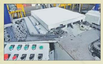
**Diamond Delta** ( $\Delta$ ) chains are pre-stretched more than ISO standard specification to enhance the performance in terms of fatigue and elongation.
